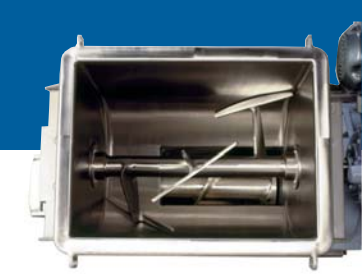
Self-feeding Hoppers eliminate product bridging and assure smooth, even feeding of raw material.
