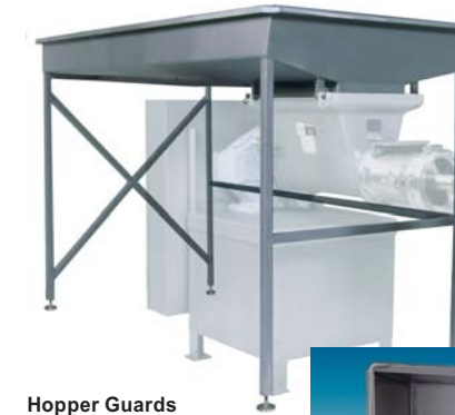
Hopper Guards accommodate standard models and most feeding methods. Custom guards are available.
