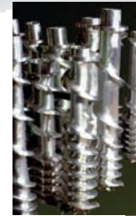
Hand-fabricated Feedscrews incorporate cupped flighting with pitches and depths to match various knife styles and applications.
